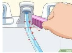
Turn on a tap of water to make a steady stream. Run a comb through your dry hair several times. Put the comb near the water and watch the water bend! This also works if you use a PVC pipe and rub it with a wool cloth or use a balloon that you rubbed on your hair.
