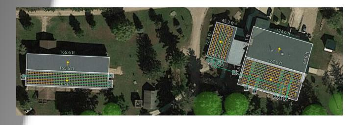
240.8kW DC ( 180KW AC) Single Phase Estimated for 80% of current consumption
